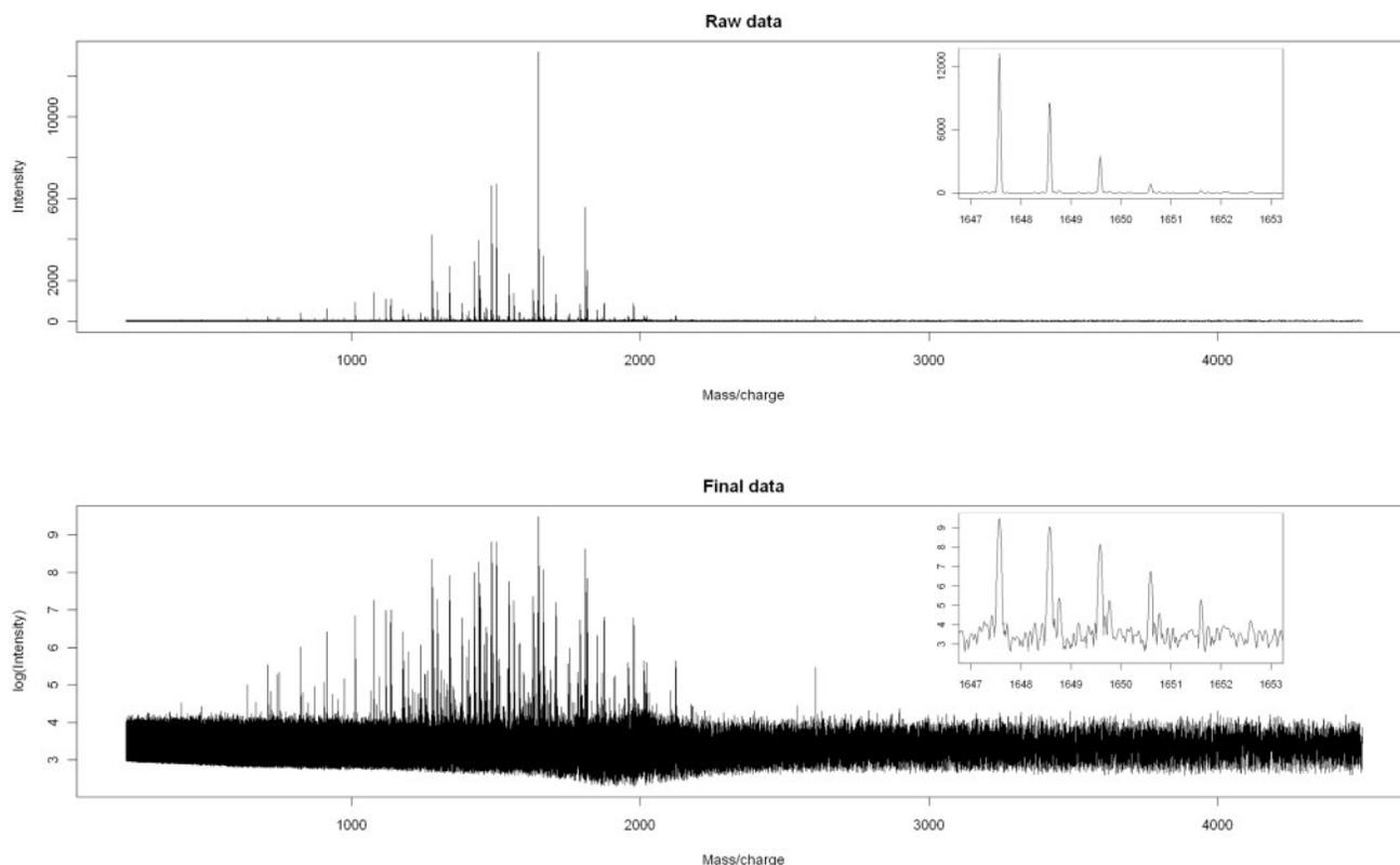
**Fig. 2.** Graphs of raw data and baseline-corrected, shifted-log-transformed data (the ‘final data’) for a typical spectrum. See Sections 2.1 and 2.2. The insets show the isotope peak sequences (see Section 4) for the most abundant compound in the spectrum.
