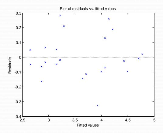
4. In an experiment to determine the factors affecting tensile strength in steel plates, the tensile strength (in kg/mm²), the manganese content (in parts per thousand), and the thickness (in mm) were measured for a sample of 20 plates. The following MINITAB output presents the results of fitting the model Tensile strength =  $\beta_0$ +  $\beta_1$  Manganese+ $\beta_2$  Thickness.
