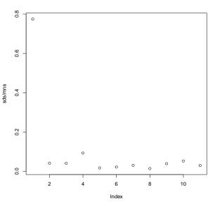
This is the ratio of the standard deviation to the mean for the 11 concentrations. The mean of the last 10 is 0.038 which is the average CV of those groups. For zero concentration, the ratio is higher as would be expected.
