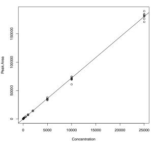
Plot of peak area vs. concentration from ICPMS along with linear calibration curve. Variance appears to increase with the mean. If the CV is nearly constant, we can take logs to stabilize the variance.
