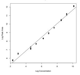
The variance no longer seems to rise with the mean. We can confirm this with a plot of the variance vs. the mean of each non-zero concentration.
